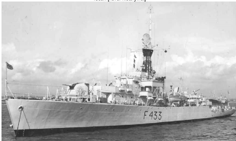
HMS Loch Insh was one of the seven Loch Class modernised in the 1950's for service in the Mediterranean Sea, the Middle East and the Far East. They took the pressure off more modern frigates allowing them to attend to responsibilities with NATO in the Atlantic. Note the black ball at the yardarm signifying that she is at anchor. [leithbuiltships.blogspot.com.au]
