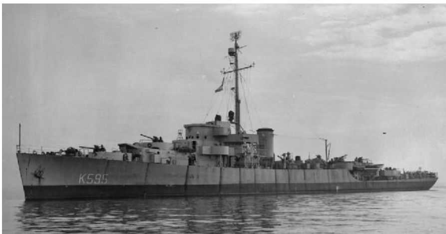
HMS Tortola . Note the American SA and compact SL radar antennae on the mast and the cross-shaped TBS antennae on the yardarm. Also, the complete absence of portholes/scuttles in the hull. [navsource.com]
