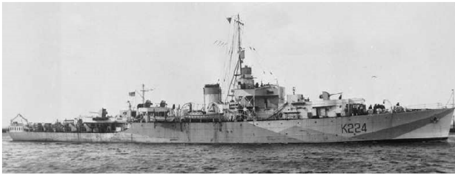
HMS Rother was completed with two single QF 2-pounder MK VIII's at the break of the forecastle but was completed without Hedgehog. [photoship.co.uk]
