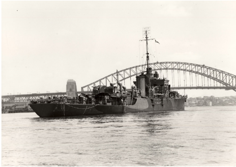
HMAS Gascoyne was one of eight built in Australia. Note the 4-inch guns were a single version of the Mk XVI twin. The camouflage pattern predates the USNs overall dark blue which became standard. The masthead radar antenna is the Australian-designed and built A286, not the American SC as often attributed. [navy.gov.au]
