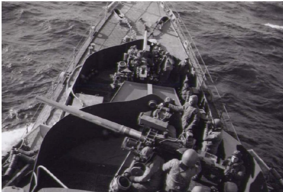
The Captain Class introduced the much-derided 3"/50 cal Mk 20-22 to Royal Navy service. This photograph is of a USN DE. [usslater.org]
