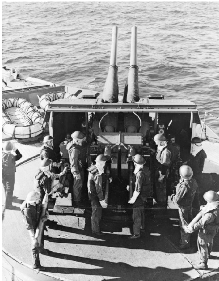
A twin QF 4-inch Mk XVI on an HA/LA Mk XIX mounting which was the mainstay of the Bay Class. Shells had to have their fuses set at the fuse-setters located to the extreme left and right-hand sides of the mount before they could be loaded. In anti-aircraft mode, the predictor had to allow for the speed of the aircraft, its course, the time to set the fuses, the time to load the shell, the time to fire, the time of flight of the projectile to the determined altitude in order to have a chance of success – which was rare. [commons.wikimedia.org]
