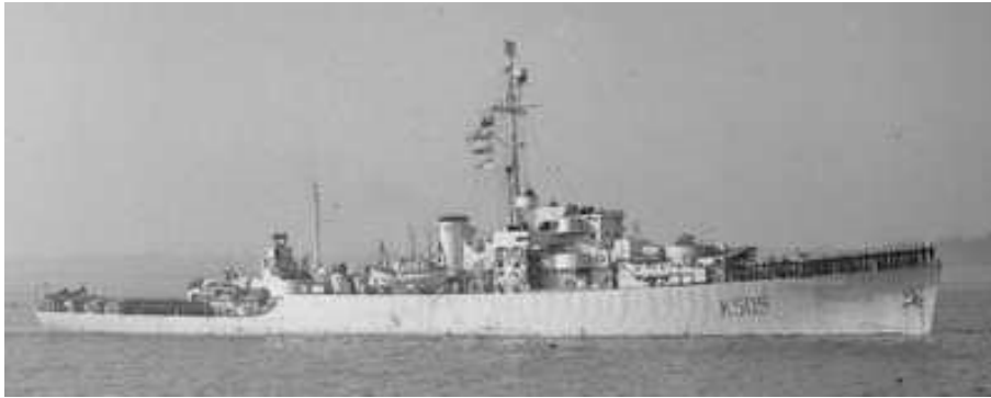
HMS Caicos converted to a Fighter Direction Ship, specifically to detect German V-1 missiles launched from the Netherlands. Note the Type 277 radar antenna, folded flat, aft of a mainmast presumably holding other warning equipment. [commons.wikimedia.org]
