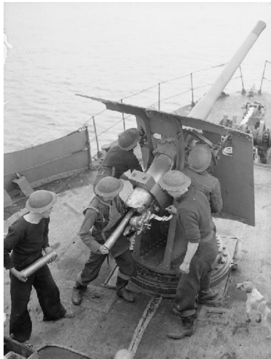
The versatile QF 12-pounder 12 cwt gun in action in anti-aircraft mode. Note that this is obviously a training exercise: the dog on the right and the shell minus projectile on the left. [commons.wikipedia.org]
