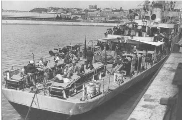
The stern of the River Class frigate HMS Parret at Port Elizabeth, South Africa. Note the slotted smoke generators, the extra 20mm Oerlikons on the quarterdeck and the ready-use racks for depth charges beside the four depth charge throwers. [navsource.org]
