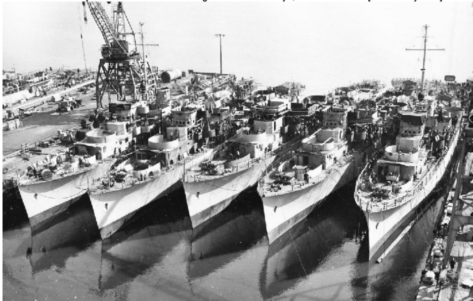
Colony Class frigates under construction. Note the long, narrow bridge above a wheelhouse with seven prominent ports. The considerable flare to the bows contributed to the seakeeping qualities of the River Class and the derivatives. [navsource.com]
