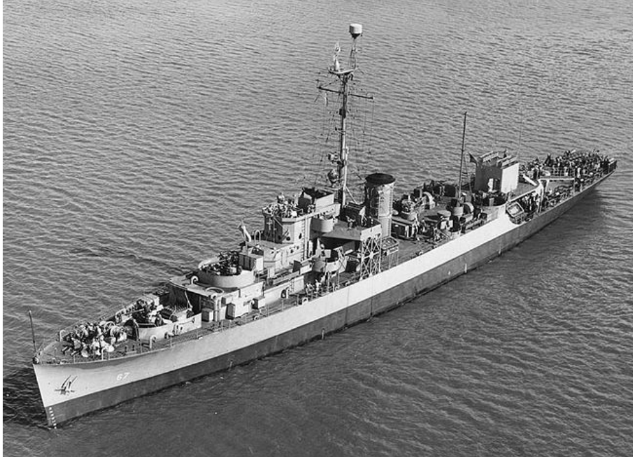
USS Peoria , a Tacoma Class Patrol Frigate converted to a weather ship but still in the two-tone camouflage. The hangar replaced the aft 3"/50 cal mount and was used for weather balloons. Note that the anchors are a fabricated Danforth type and deck vents are simple goosenecks – all to simplify and speed production. [photoship.co.uk]
