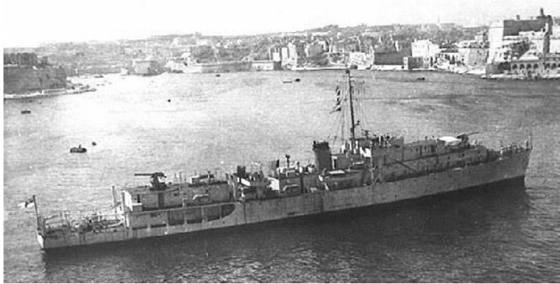
HMS Derby Haven as a depot ship for coastal forces. Note the QF 4-inch Mk V mounts fore and aft. Note the simple pole mast with what looks like an American SG radar. [naval-history.net]
