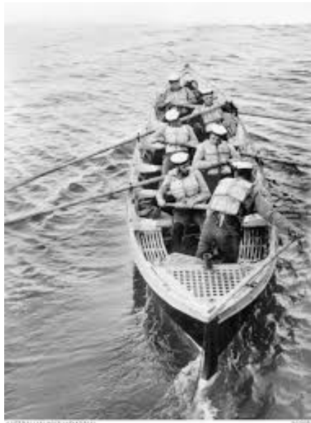
A 27-foot Montagu from the Tribal Class destroyer HMAS Warramunga pulling away from the ship's side, Korea 1952. Note the coxswain is using a direct tiller to the rudder head and not a tiller mounted forward of the mizzen mast, the support for which is clearly visible. [Australian War Memorial]
