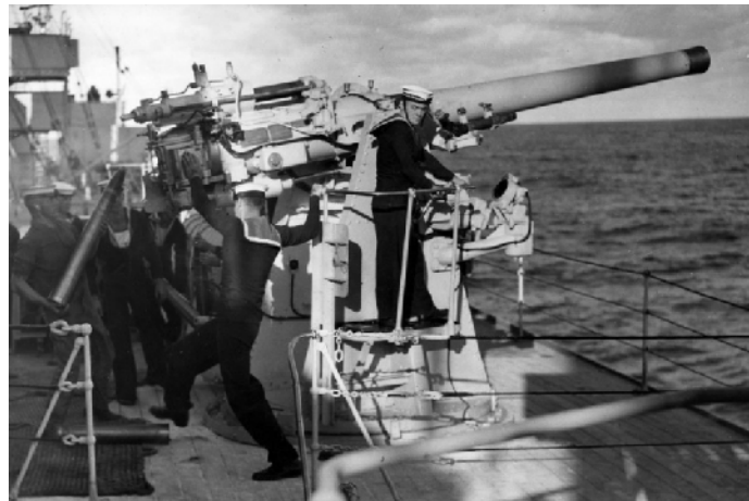
The Loch Class introduced a shielded version of the QF 4-inch Mk V – shown here on HMAS Canberra . Note how tall the mount is in order to achieve the elevation for it to be an effective anti-aircraft weapon. [State Library of Victoria: H98.105/3227]
