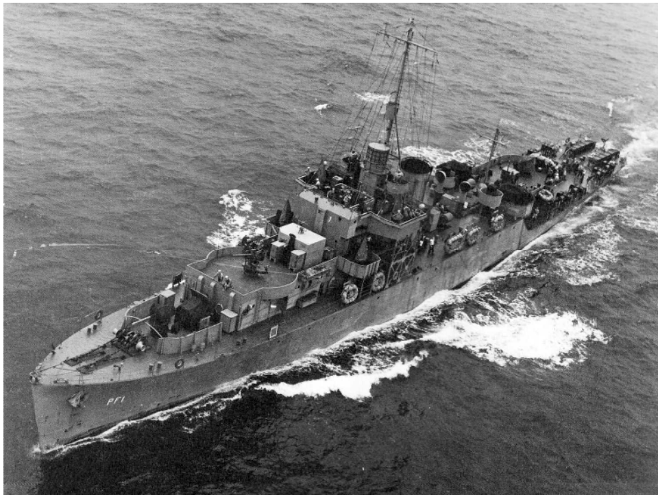
The United States Navy's Patrol Frigate Asheville , transferred from the Royal Navy in a reverse Lend Lease in December 1942. In effect a River Class frigate with American armament. Note that there are no 20mm Oerlikons fitted amidships like the Tacoma Class. [navsource.org]
