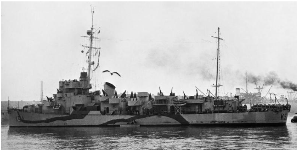
HMS Lawford converted to a Landing Ship Headquarters (Small) LSH (S). Note that she still has her full complement of depth charges in rails at the stern. Also, the small boat alongside, below the torpedo-loading davit that has been installed, is probably the “skimmer” or runabout reported as having been carried. [photoship.co.uk]
