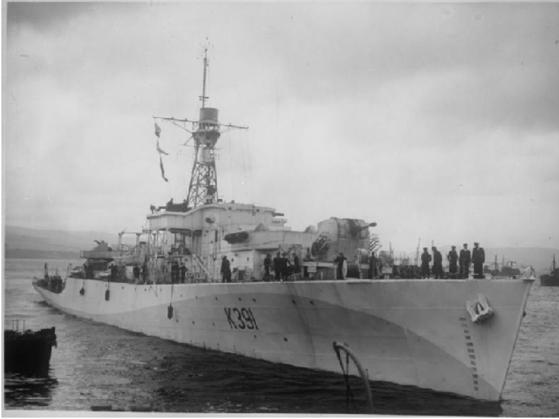
Killer of three U-Boats, HMS Loch Killin returning to port. Note the three economy-measure straight lines in the sheer. The radar atop the lattice mast is not yet the Type 277 it was designed for but a variant of the Type 271 – possibly Type 271Q or 272. A Type FH 4 HF/DF antenna is just visible at the masthead. The camouflage scheme is basically an all-white hull with a lower flash of Western Approaches Green or Blue – both very pale colours. [commons.wikimedia.org/wikivisually.com]
